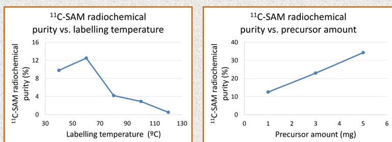
Figure 3: Variations of <sup>11</sup>C-SAM radiochemical purity in the reaction mixture with different labelling temperatures and precursor amounts.
