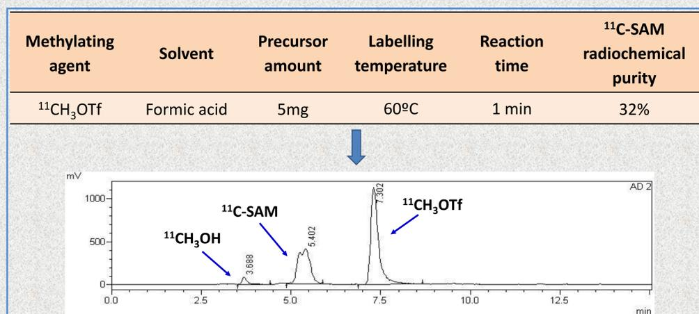
Figure 4: Optimum labelling conditions and gamma chromatogram of the reaction mixture.
